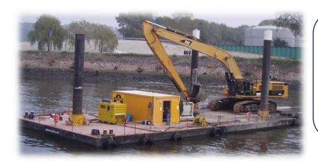
For rock excavation, we can implement a CAT excavator on a modular barge equipped with spuds. The dimensions of the barge are adapted in function of the project and full stability analysis is realized and approved by Bureau Veritas.
